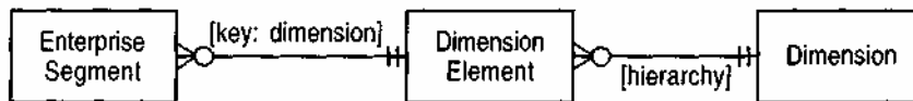
Figure 4.4 Defining enterprise segments by using dimensions and dimension elements. This model allows us to add new dimensions without changing the model. It is also more compact.
