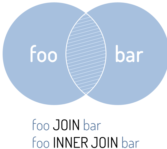
Figure 4.1. INNER JOIN behavior illustrated as a Venn diagram.
